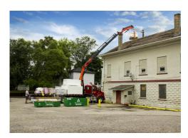
PALFINGER offers a variety of cranes specifically suited for the roofing delivery industry. Knuckle boom cranes are designed for precise product placement. Ease of maneuverability allows for spreading materials along a roof. These machines eliminate the need to handle product on the ground and reduce the number of workers needed for deliveries. The compact design and low weight of these cranes give delivery companies the ability to carry increased payload.
