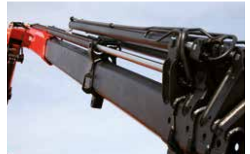
LOW-MAINTENANCE EXTENSION SYSTEM REDUCES SERVICE TIME
