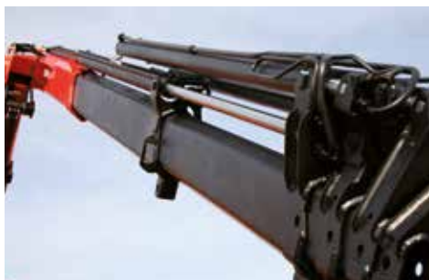
LOW-MAINTENANCE EXTENSION SYSTEM REDUCES SERVICE TIME
