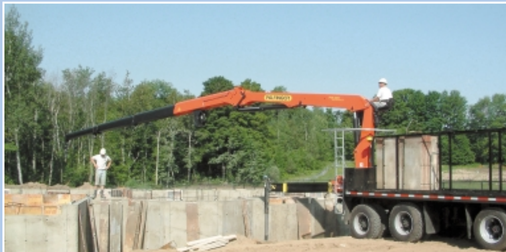
PowerLink™ linkage system gives the outer boom added strength in flat-out position and a constant folding speed.
