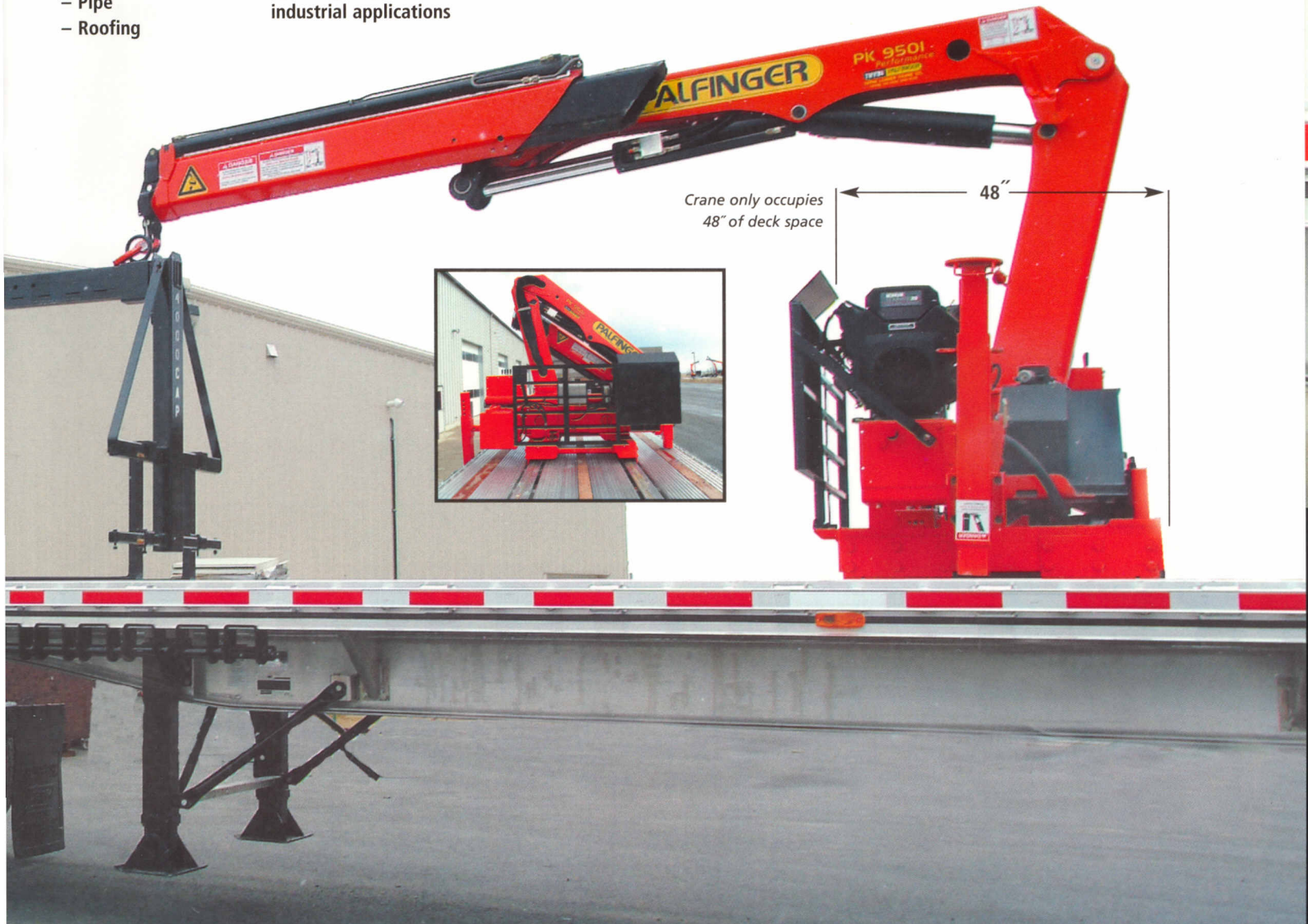
The PALFINGER crane travels the full length of the flatbed
