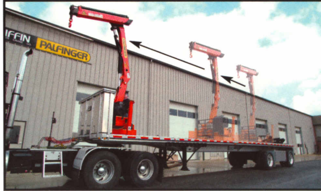
The PALFINGER crane travels the full length of the flatbed
