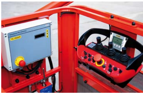
EMERGENCY SHUT-OFF BUTTON AND PROTECTED HANDRAIL OPTIMUM PROTECTION ON THE WORKMAN BASKET
