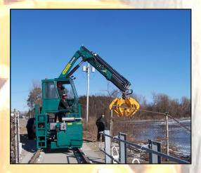
The *Debris Loader* manufactured by Tiffin Loader Crane is the ideal solution for lifting, loading, and clearing any and all types of debris. All movements are controlled by self-contained in-cab controls or by a radio remote handset. The *Debris Loader* has been a proven time-saver and greatly reduces the risks of accidents while working. Please contact us for more information and pricing at (419) 448-8156 or email us at sales@tiffincrane.com
